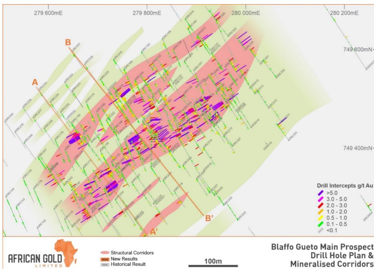
Figure 3: Blaffo Gueto Prospect Plan showing drill traces and intercepts and high-grade corridors within a broader lower grade system.
